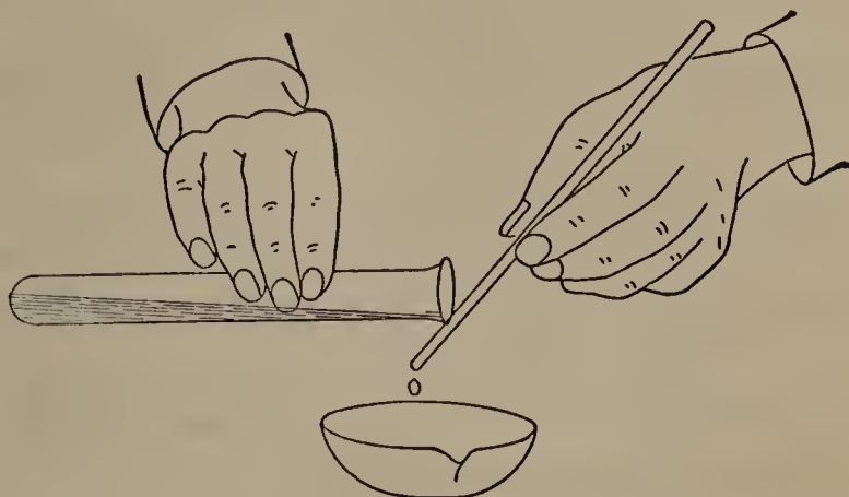
Fig. 43. Neutralizing a base with an acid.
